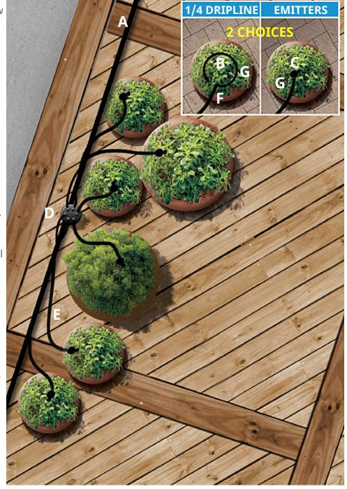
**G- 1/4" Tubing Stake** Use the tubing stakes to hold drip heads and tubing at the desired height. These stakes are universal and will work with all drip systems (part # DR-10402-65721).
