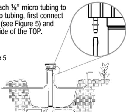
5. Use the rubber caps provided to close all unused outlets. Do this by removing the cover and the Mini-Disk filter. Press the rubber caps into the unused outlets. Re-install the Mini-Disk filter and cover. Tighten cover by hand.
