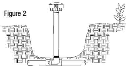
3. Excavate a narrow path to a depth of 4" from each individual plant to the TOP and lay out micro tubing within the trenches or leave micro tubing above ground and cover with mulch.
