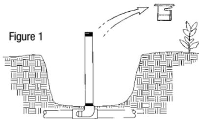
2. After the line has been flushed, thread the TOP onto the riser.
